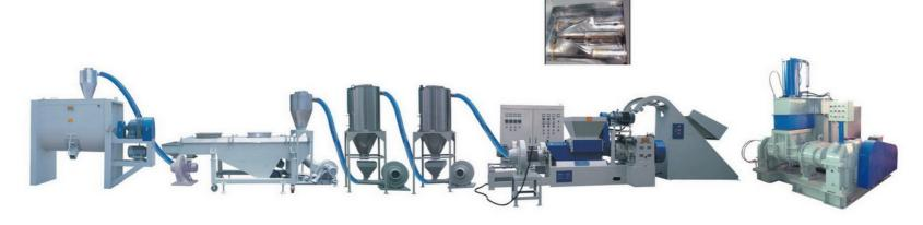
此機臺用於PVC, EVA, TPR等塑膠原料的生產,包括主機,雙腕入料,模頭切粒等系統 將密煉機攪拌好的原料經雙腕擠入造粒機內 經螺桿擠出切成粒子,此機臺操作簡單。 This machine is normally used to produce PVC, EVA and TPR raw material. It consists of main body, -shaft feeder and die-face cutting system etc. Put the mixed material into the feeding inlet. After being pushed in by two shafts, the material is extruded by a screw. The granules which being out the final product. This machine is easy to operate.
